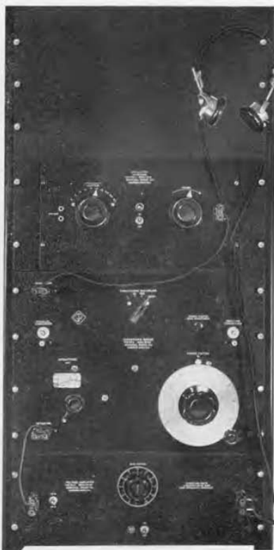
FIGURE 6. Showing how the bridge can be mounted in a relay rack with TYPE 508-A Oscillator and TYPE 714-A Amplifier
